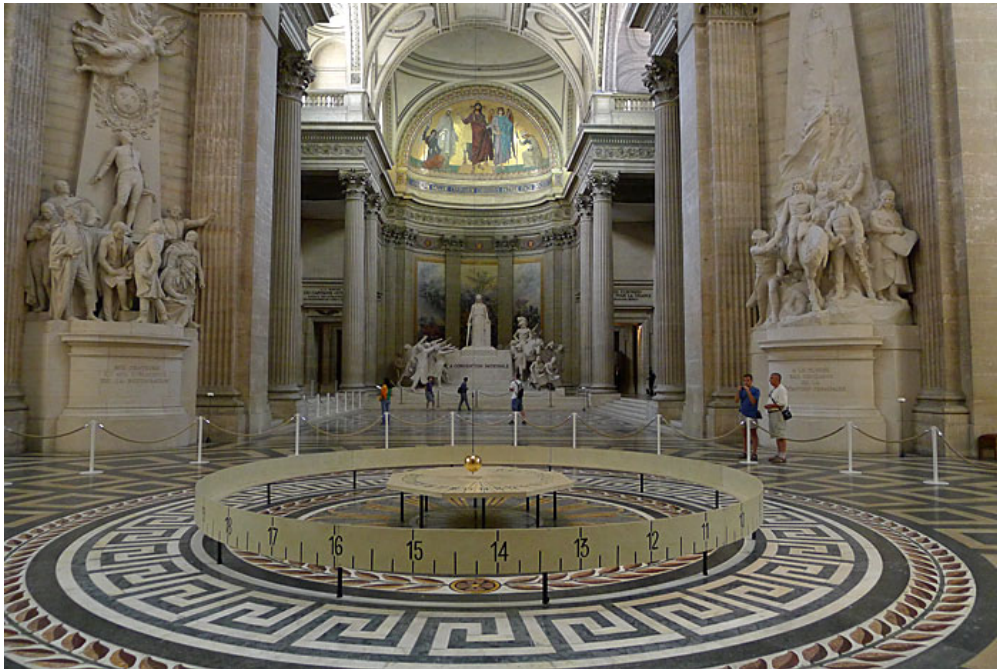
Figure 1.4: Foucault's famous pendulum in the Pantheon, Paris. What keeps it moving? Air resistance would normally stop the pendulum after a few hours – so an iron collar is installed on the wire surrounded by an electromagnet that attracts the collar as the bob swings out, then shuts off automatically as it swings back, thus, keeping pendulum going. The magnet is turned on and off by a switch which is activated when the support wire interrupts a beam of light shining across its path. Similar idea is followed by the Bremen Foucault's pendulum in our department.
