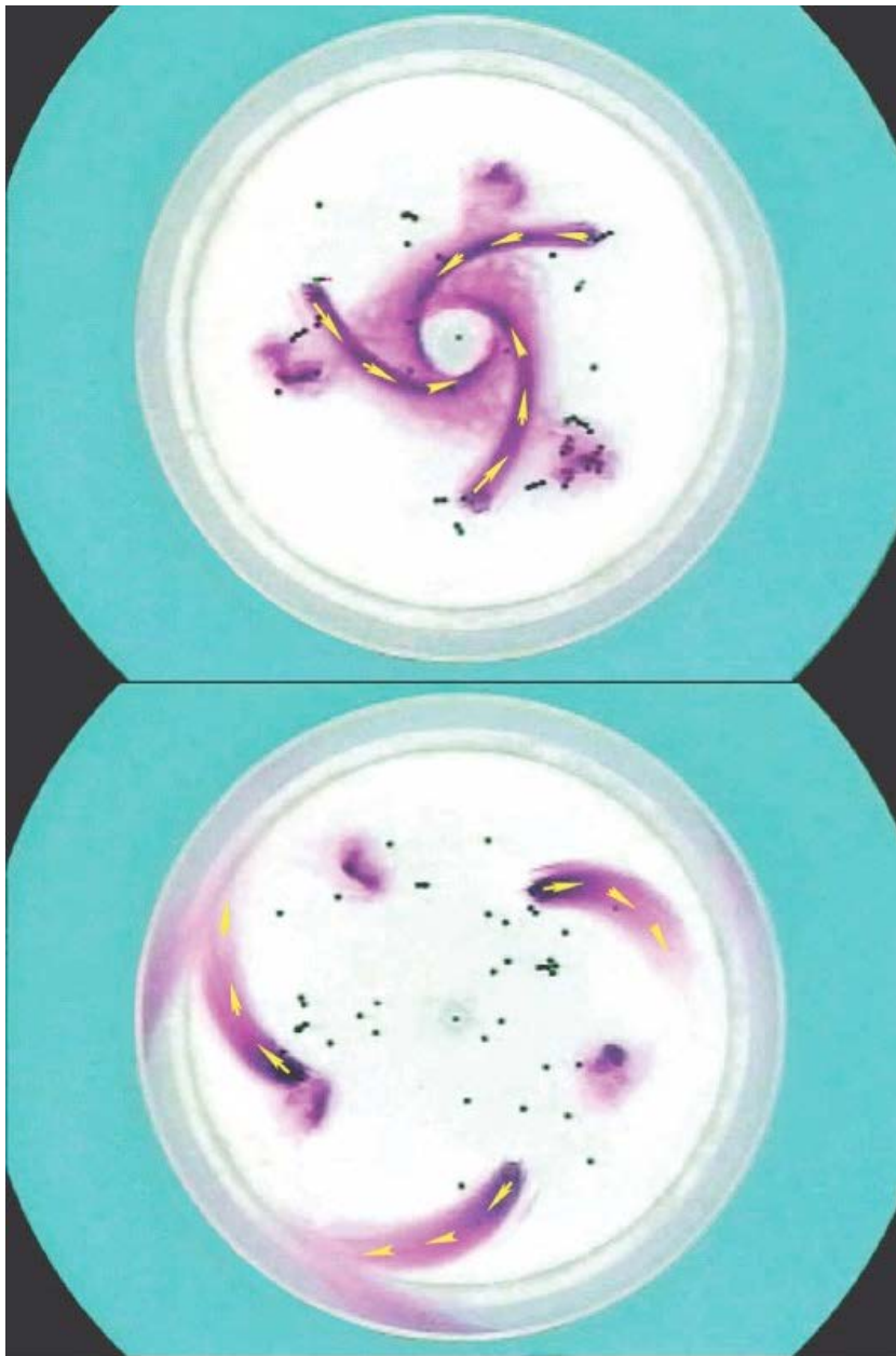
Figure 6.16: To carry out the experiment we first very slightly reduce (by 10% max) the rate of rotation of the turntable. Because of the inertia of the turning fluid, it continues to spin at its original speed and so moves relative to the tank: permanganate streaks are pulled around not in circles as one might initially expect, but rather inward turning, anticlockwise spirals, as can be seen in the top panel. A beautiful symmetric pattern is remarkably easy to achieve. This is analogous to the near-surface flow in a low pressure system, as can be seen by comparing with Fig. 4.2 (see low pressure system). To visualize the flow at the upper surface, we can float a few paper dots on the surface (black dots are the most visible in this application). We observe circular, rather than spiraling, motion. To create an analogy of a high pressure system we now simply increase the speed of the turntable by 10% or so (back up to, roughly, its original speed). We observe the dye streaks on the bottom reversing and, over time, spiraling clockwise and outwards, as can be seen in the lower panel in this figure. This should be compared to the pattern of surface winds that can be seen in the high pressure system in Fig. 4.2. From Marshall and Plumb (2007).
