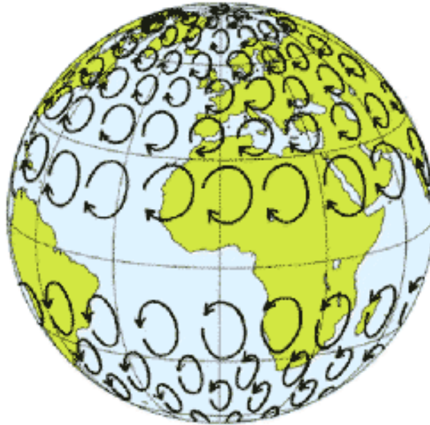
Figure 7.4: Schematic representation of inertial circles of air masses in the absence of other forces, calculated for a wind speed of approximately 50 to 70 m/s. Note that the rotation is exactly opposite of that normally experienced with air masses in weather systems around depressions.
