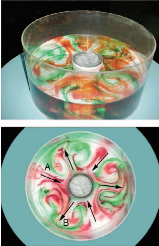
FIGURE 8.7. Top: Baroclinic eddies in the “eddy” regime viewed from the side. Bottom: View from above. Eddies draw fluid from the periphery in toward the centre at point A and vice versa at point B. The eddies are created by the instability of the thermal wind induced by the radial temperature gradient due to the presence of the ice bucket at the center of the tank. The diameter of the ice bucket is 15 cm.
