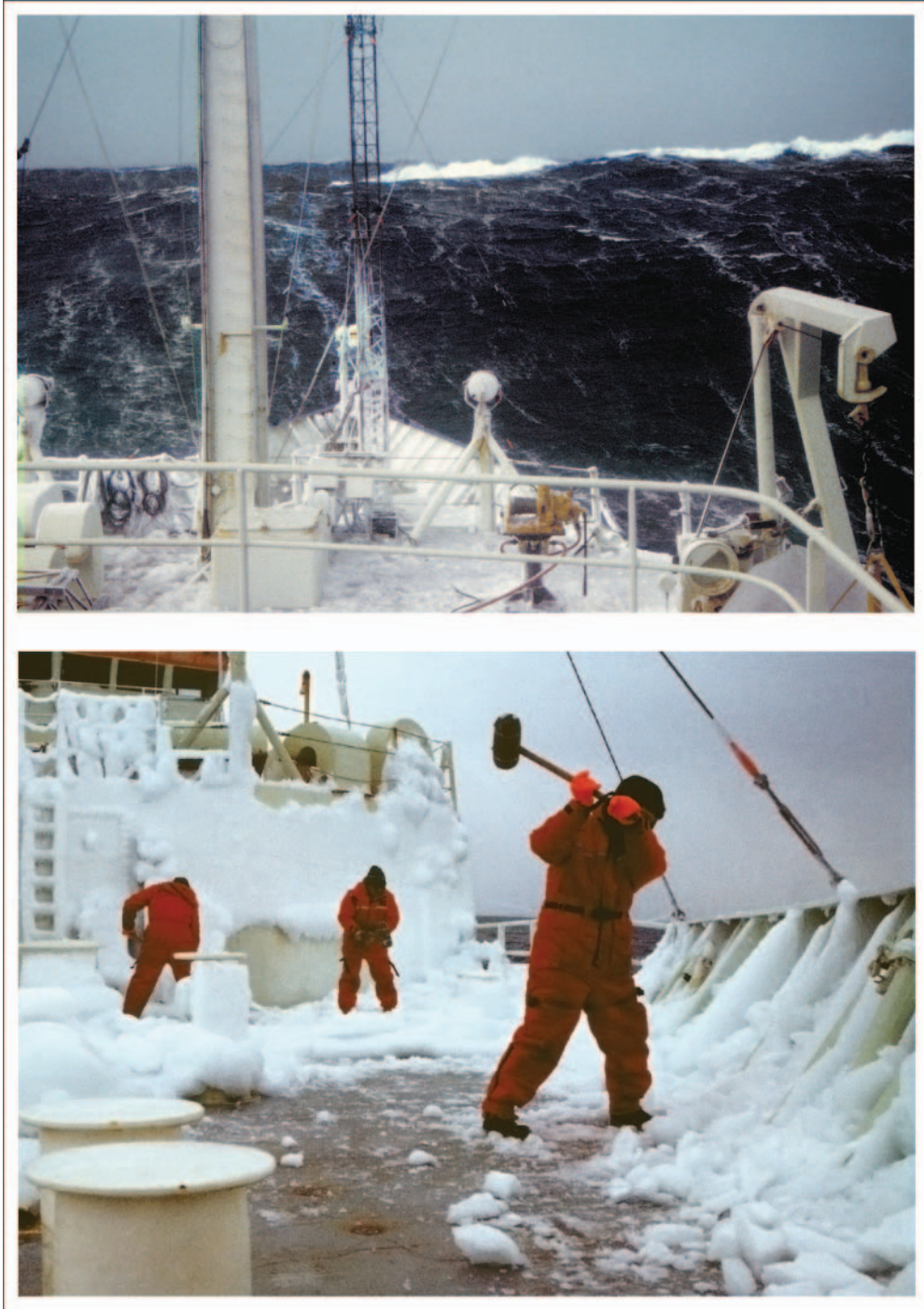
FIGURE 11.10. The Woods Hole ship KNORR cuts through harsh Labrador Sea conditions during the winter Labrador Sea Deep Convection Experiment (Feb–Mar, 1997) taking observations shown in Fig. 11.11. Waves such as those shown at the top caused continual ice build-up on the ship, as can be seen at the bottom. Courtesy of Bob Pickart, WHOI.
