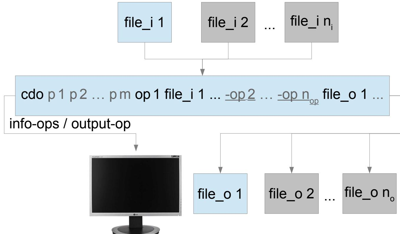
input files `file_i`, output files `file_o`, program options `p`, operators `op1`; grey: optional;
