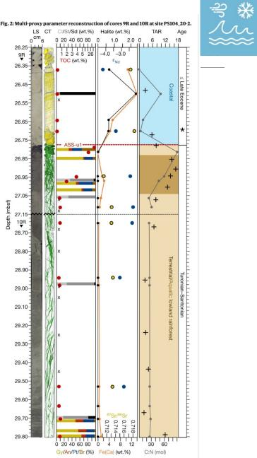
The MARUM-MeBo70 seafloor drill rig drilled 30.7 m into the seafloor and recovered 5.91 m of core length. The lower -3 m consists of a fossil root-bearing mudstone with an -5-cm-thick layer of brecciated lignite on top (from -26.77 mbsf downwards), both of Turonian–Santonian age. A Late Eocene or younger quartzitic gravelly sandstone overlies the lignite. The upper lignite boundary defines the impedance contrast between the
