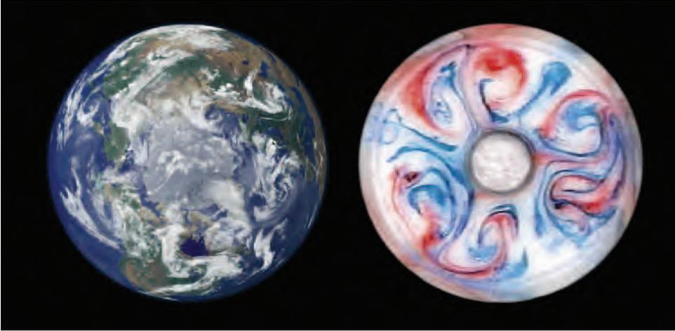
**FIGURE 6.1.** Throughout our text, running in parallel with a theoretical development of the subject, we study the constraints on a differentially heated, stratified fluid on a rotating planet (left), by using laboratory analogues to illustrate the fundamental processes at work (right). A complete list of the laboratory experiments can be found in Appendix A.4.
